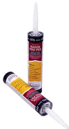
Pro PGS meets radon standards and is the ideal sealant for most basement and crawlspace needs. Use limestone-colored, non-yellowing Pro PGS for sealing expansion and control joints (i.e., wall joints, window and door perimeters, copings, etc.). This easy-to-use, professional-grade polyurethane sealant is self-leveling, long-lasting, non-sag, flexible, and moisture-curing.
