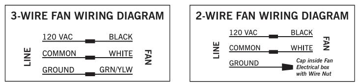
Note: Some of our fan models use motors that do not utilize a ground wire. This wire configuration is safe and allowable under our ETL safety listing. If the fan being installed was constructed with the 2-wire configuration (no ground), the ground wire from the Line supply should be capped with a wire nut inside the electrical box at the fan.
