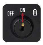
• **ON** – Device is on, hardware buttons can be used and Bluetooth will work while key switch in ON position.
