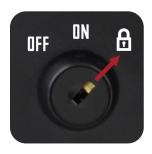
• LOCK – In the lock position, the buttons on the RadStar are disabled. Insert key, turn to LOCK position, and then REMOVE KEY. Bluetooth will work while key switch is in LOCK position.
